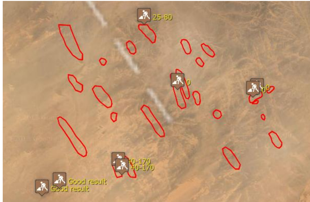
Fig. 1. The anomalies we identified are shown in red. The symbols indicate the sampling zones with approximate gold grades in g/t (grams per ton).
